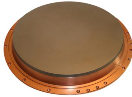
FIG. 5. Left: EDX of the pressed ceramic \text{PbZr}_{0.52}\text{Ti}_{0.48}\text{O}_3 Right: Custom formulation lead oxide saturated (1-x)\text{PbZr}_{0.52}\text{Ti}_{0.48}\text{O}_3 + x\text{PbNdO}_3 target, D=300 mm, bonded to a Cu backing plate.
