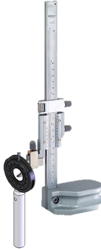
Figure 3.5. Vernier height gauge used to set up the irises in the optical path.
