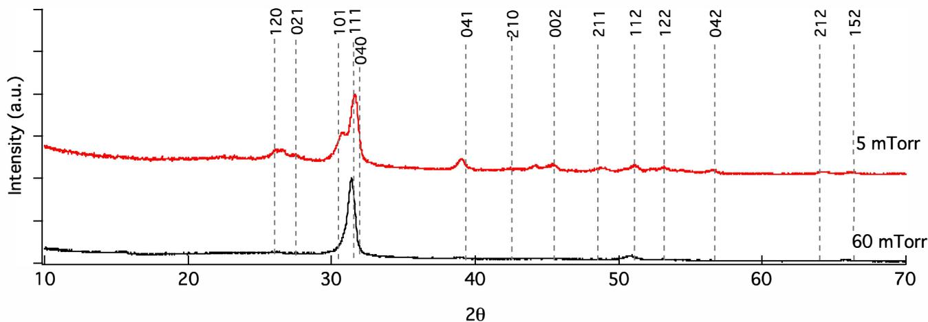
Fig. 4. X-ray diffraction patterns of SnS films deposited at 5 and 60 mTorr total pressure and 105 W target power. Pattern data are matched to PDF# 39-354.
