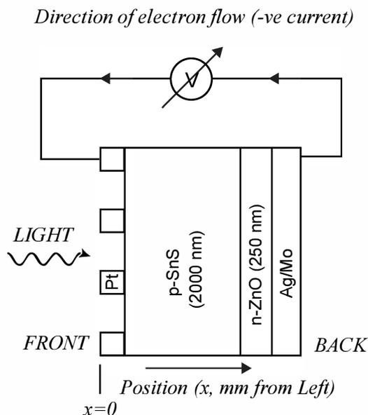
Fig. 1. Schematic of SnS|ZnO solar cell in the substrate configuration. Schematic is for a 1-D model used to predict the efficiency of a SnS|ZnO heterojunction solar cell, with light impinging from the left.
