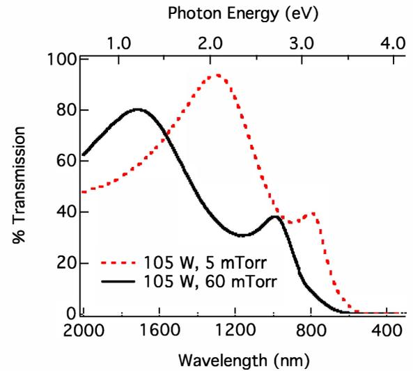
Fig. 7. Transmission spectra for SnS films grown on glass slides.
