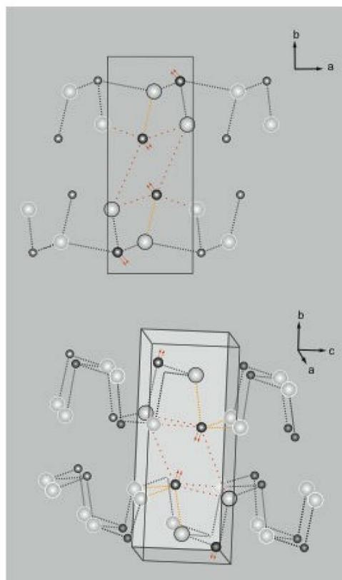
Fig. 5. Structure of SnS. (Top) cross section of the  $b$ -zone axis (Bottom) 3-D unit cell projection of the  $c$  zone axis (unit cell tilted). Dark and light spheres represent tin and sulfur atoms, respectively (unit cell: outlined in black). Dashed lines are covalent bonds.
