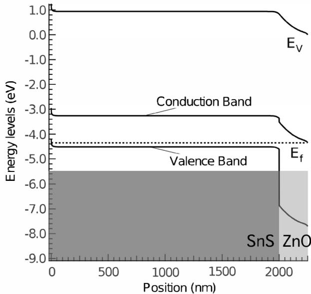
Fig. 2. Predicted Energy Band Diagram for the SnS/ZnO materials system from AMPS-1D modeling program. In this setup, light would enter from the left side. Electron flow is to the right.  $E_v$  is the vacuum level and  $E_f$  is the Fermi level.
