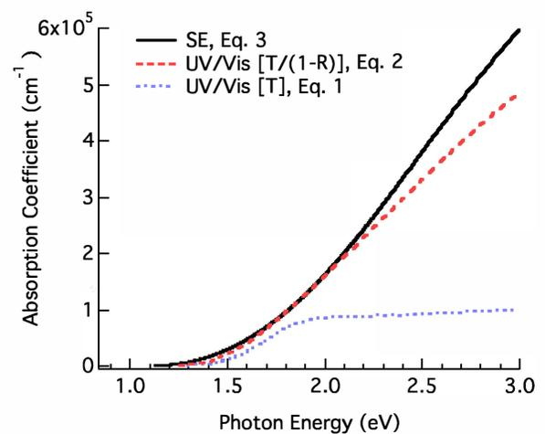
Fig. 8. Absorption coefficient ( $\alpha$ ), obtained from spectroscopic ellipsometry analysis and ultraviolet-visible spectrophotometry for an SnS film prepared at 135 W target power and 60 mTorr total pressure.
