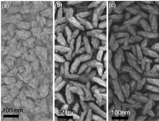
Fig. 6. Field emission scanning electron microscopy images of SnS material deposited at (a) target power 105 W, 5 mTorr total pressure; (b) target power 115 W, 10 mTorr total pressure; and (c) target power 145 W, 10 mTorr total pressure.
